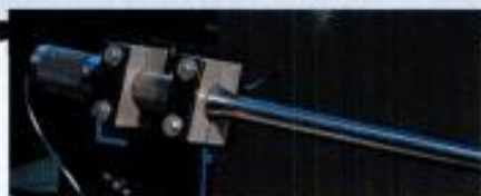
No more snip-and-run: The PAN disrupter's shock tube can be as long as 5,000 feet for remote use.
