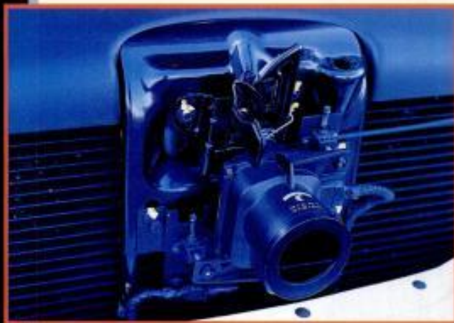
The infrared camera is mounted on the front of the radiator, facing forward. Everything but the lens is covered by the grille.
