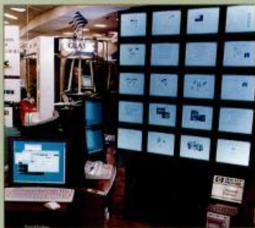
Demonstrated at a recent trade show, the PixelVision video wall is constructed from 20 separate LCD panels.
